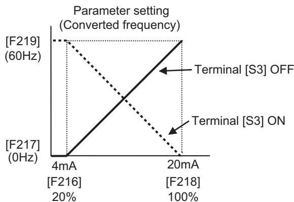
\* When switching the characteristics using terminals, not only characteristics of set value but also of feedback value switches.
