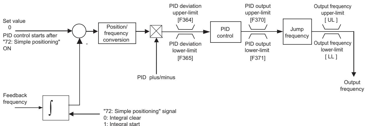
\* While the [72: Simple positioning] signal is not input, the PID control is not executed.
