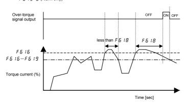
When  $F \mathcal{B} \mathcal{B} = \mathcal{B}$  (tripping), the inverter will trip if over-torque lasts for the period of time set with  $F \mathcal{B} \mathcal{B}$ . In such a case, the over-torque signal remains ON.
