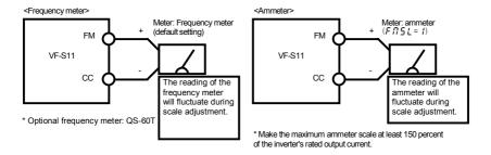
[Example of how to adjustment the FM terminal frequency meter]
