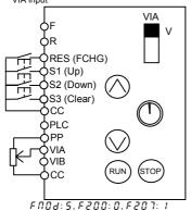
F ! ! 3: 38 (Allocation of FCHG) To switch to VIA setting, enter the command through FCHG.
