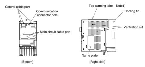
Note 1) Remove this seal when installing the inverter side by side with other inverters where the ambient temperature will rise above 40°C.
