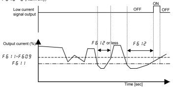
\* When setting F & I : To I (Trip), trip after low current detection time setting of F & I : After tripping, the low current signal remains ON.
