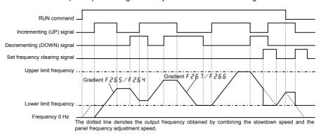
Note: If the operation frequency is set to the lower limit frequency, it will increase from 0Hz when power is turned on for the first time after the setting, and therefore the output frequency will not rise until the operation frequency reaches the lower limit frequency. (Operation at the lower limit frequency) In this case, the time required for the operation frequency to reach the lower limit frequency can be shortened by setting fc to the lower limit frequency.
