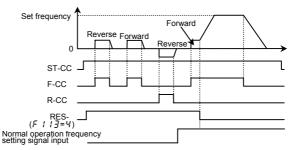
The jog run setting terminal (RES-CC) is enabled when the operation frequency is below the jog run frequency.
