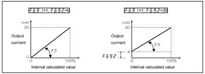
Note 1) When using the FM terminal for current output, be sure that the external load resistance is less than  $750\Omega$ . Note 2) Note that, if  $F \Pi S L$  is set to T (torque), data will be updated at intervals of more than 40 ms.
