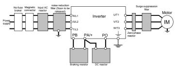
Note 1: The T/L3 terminal is not provided for any single-phase 240V model. So if you are using a singlephase 240V model, use the R/L1 and S/L2 terminals to connect power cables.
