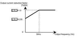
Note: The motor overload protection start level is fixed at 30Hz.
