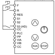
Selecting HD (operation holding) with the input terminal selection parameter
