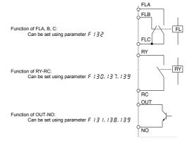
■ Assigning one function to an output terminal
