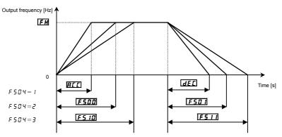
Acceleration/deceleration time 1 is initially set as the default. Acceleration/deceleration time 2 and 3 can be selected by changing the setting of the  $F \in \mathcal{G} \cup \mathcal{G}$ . Enabled if  $f \in \mathcal{G} \cup \mathcal{G} \cup \mathcal{G}$  (panel input enabled)
