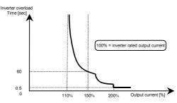
To protect the inverter, overload trip or overcurrent trip activate in a short period of time when output current reaches 150% or higher.
