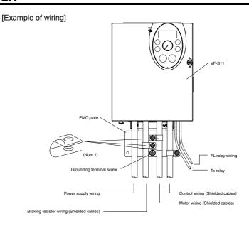
Note 1: Strip and earth the shielded cable, following the example shown in Fig.
