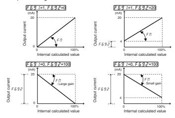
★ The analog output inclination can be adjusted using the parameter F \(\overline{I}\).
