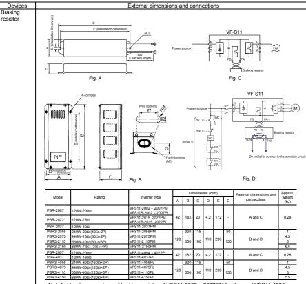
Note1: Use the same type of braking resistor of VFS11-2002 ~ 2007PM for those of VFS11-4004 ~ 4022PL.
