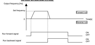
[F 10 5 = 0 (Reverse)]: If an F command and an R command are entered simultaneously, the motor will run in the reverse direction.
