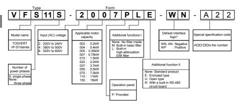
\* This code represents the factory default logic setting. You can switch from one input/output logic to the other using slide switch SW1. (See 2.3.2)
