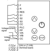
To switch to preset-speed setting, use the external terminals S1 to S3
