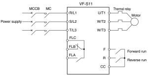
Example of connection of a magnetic contactor in the primary circuit
