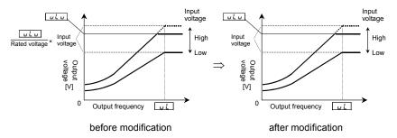
In case of F 3 0 7=2 [ Supply voltage uncorrected, output voltage unlimited]
